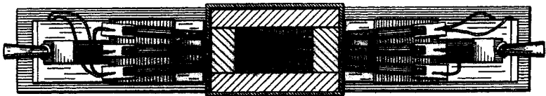
FIG. 2.—Plan View of Furnace with Cover Removed.
